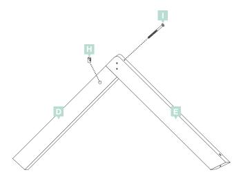
Join x1 Short Arm D to x1 Long Arm E using x1 Long Bolt D and x1 Barrel Nut H. Repeat for remaining Short Arm D and Long Arm E.
