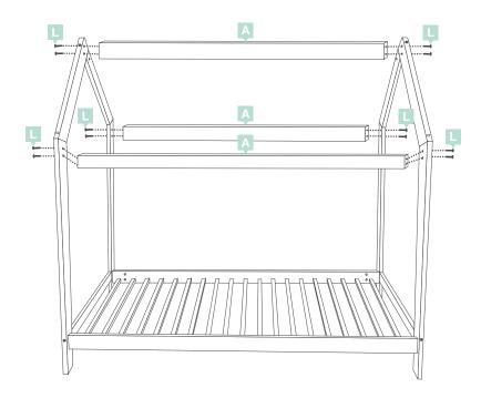
Complete assembly of your Harper Toddler Bed House by joining x3 Long Panels A to Step 4 using x12 Conformats L.
