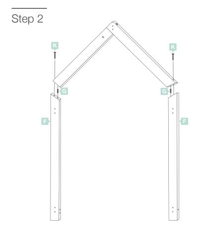
Join x2 Legs F to Step 1 using x2 Dowels G and x2 Conformats K.
