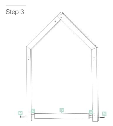
Join x1 Short Panel B to Step 2 using x2 Dowels G and x2 Conformats M.
