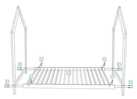
Join Base C to both parts of Step 3 using x8 Short Bolts J and x8 Barrel Nuts H.
