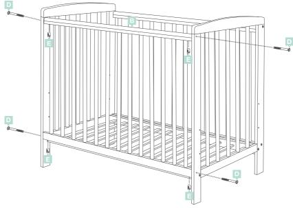
Complete assembly of your Compact Cot by joining the remaining Side Rail with x4 Bolts and x4 Barrel Nuts.
