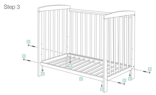
Join Compact Cot Base C to Step 2 at the required height with x4 Bolts D and x4 Barrel Nuts E.
