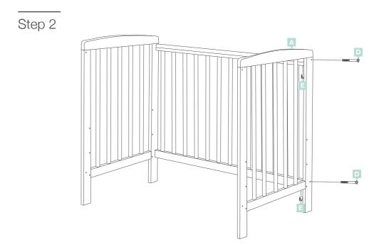
Join remaining Compact Cot End A to Step 1 with x2 Bolts D and x2 Barrel Nuts E.
