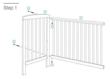
Join Compact Cot End A to Side Rail B with x2 Bolts D and x2 Barrel Nuts E.
